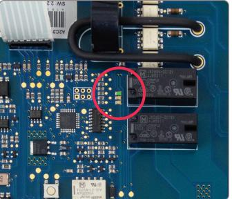
If the error has been successfully reset the **GREEN** LED on the PCB will start to flash slowly, indicating the unit is now in standby mode. You can now reconnect the display PCB cable and replace the exterior cover.
