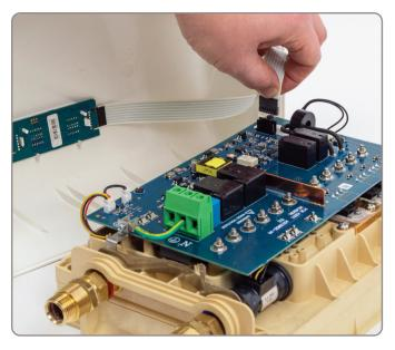
1. Remove the cover and unplug the connecting cable from the PCB.
