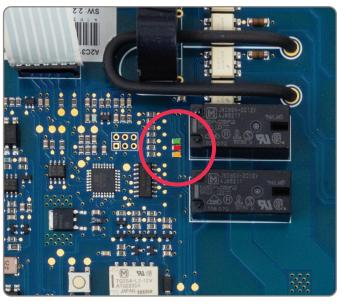
The three LED indicators on the PCB will be illuminated when the unit is in standby, running or in error mode.
